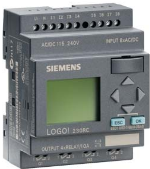
LOGO! 230RC,LOGIC MODULE,DISPL. PU/I/O: 115V/230V/RELAY, 8 DI/4 DO, MEM. 200 BLOCKS, EXPANDABLE WITH EXTRA MODULES 230V AC/DC
