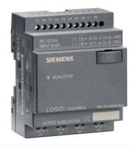
$^{\star\star\star}$  Spare part  $^{\star\star\star}$  LOGO! 12/24RCO, logic module PS/I/O: 12/24 V DC/relay, 8 DI (4 AI)/4 DO, without display, memory 200 blocks, modular expandable
