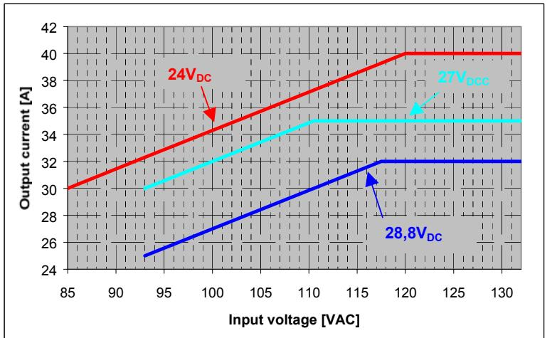
At input voltages between 85V<sub>AC</sub> and 93V<sub>AC</sub> the output voltage is limited to 24V<sub>DC</sub>.
