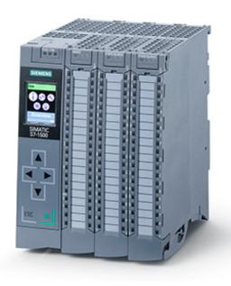
SIMATIC S7-1500 COMPACT CPU CPU 1512C-1 PN, CENTRAL PROCESSING UNIT WITH WORKING MEMORY 250 KB FOR PROGRAM AND 1 MB FOR DATA, 32 DIGITAL INPUTS, 32 DIGITAL OUTPUTS, 5 ANALOG INPUTS, 2 ANALOG OUTPUTS, 6 HIGH SPEED COUNTERS, 1. INTERFACE: PROFINET IRT WITH 2 PORT SWITCH, 48 NS BIT-PERFORMANCE, INCL. FRONT CONNECTOR PUSH-IN, SIMATIC MEMORY CARD NECESSARY
