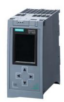
\*\*\* Spare part \*\*\* SIMATIC S7-1500, CPU 1516-3 PN/DP, central processing unit with work memory 1 MB for program and 5 MB for data, 1st interface: PROFINET IRT with 2-port switch, 2nd interface: PROFINET RT, 3rd interface: PROFIBUS, 10 ns bit performance, SIMATIC Memory Card required
