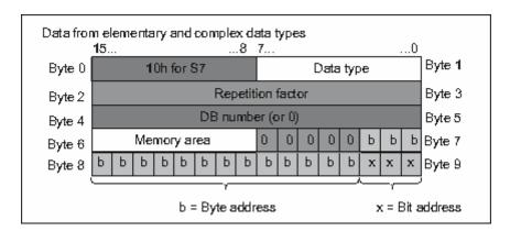
The repetition factor identifies a quantity of the indicated data type to be transferred by the parameter type ANY. This means you can specify a data area and also use arrays and structures in conjunction with the parameter type ANY. STEP 7 identifies arrays and structures as a number (with the help of the repetition factor) of data types. If, for example, 10 words are to be transferred, the value 10 must be entered for the repetition factor and the value 04 must be entered for the data type.
