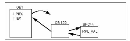
In this example, the substitute value in the following figure is entered in the program so that the program can continue to operate with feasible values.
