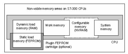
To do this set the CPU so that the following data are saved in the nonvolatile RAM:
