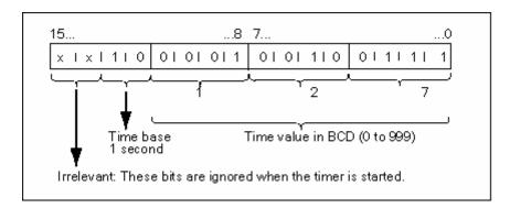
When working with S5TIME, you enter a time value in the range of 0 to 999 and you indicate a time base (see the following table). The time base indicates the interval at which a timer decrements the time value by one unit until it reaches 0.
