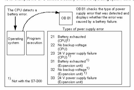
You can write a program that evaluates the event code triggered by the OB81 call. You can also write a program that brings about a reaction, such as activating an output connected to a lamp on the operator station.
