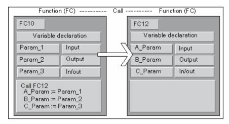
STEP 7 restricts the assignment of formal parameters of an FC as actual parameters for the formal parameters of a different FC. You cannot, for example, assign parameters with complex data types or a parameter type as the actual parameter.
