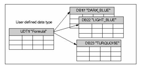
The structure of the data block is determined by the UDT assigned to it.
