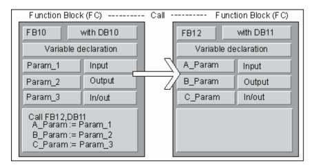
STEP 7 restricts the assignment of the formal parameters of an FB to the formal parameters of another FB. You cannot, for example, assign input and output parameters with complex data types as the actual parameters for the input and output parameters of a called FB. You can, however, assign input parameters of the parameter types TIMER, COUNTER, or BLOCK to the input parameters of the called FB.
