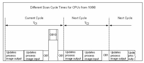
In the current cycle, OB1 is interrupted by a time-of-day interrupt.
