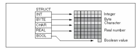
A structure can be nested to a maximum of 8 levels (for example, a structure consisting of structures containing arrays).
