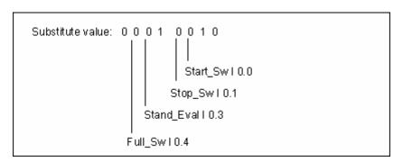
If an input module fails, the processing of the statement L PIB0 produces a synchronous error and starts OB122. As standard, the load instruction reads in the value 0. With SFC44, however, you can define any substitute value suitable for the process. The SFC replaces the accumulator content with the specified substitute value.
