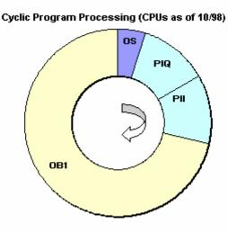
One of the internal tasks of the operating system (OS) is to write the process image output table (PIQ) to the outputs for the modules and to read in the status of inputs into the process image input table (PII). Once this step is complete, the user program is executed with all blocks that are called
