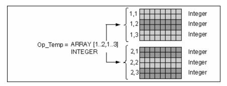
You access the data in a multi-dimensional array using the index. In this example, the first integer is Op\_temp[1,1], the third is Op\_temp[1,3], the fourth is Op\_temp[2,1], and the sixth is Op\_temp[2,3].
