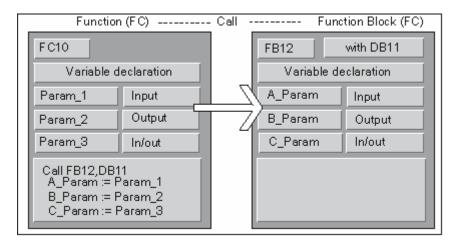
STEP 7 restricts the assignment of formal parameters of an FC to the formal parameters an FB. You cannot, for example, assign parameters with a complex data type as actual parameters. You can, however, assign input parameters of the parameter types TIMER, COUNTER, or BLOCK to the input parameters of the called FB.
