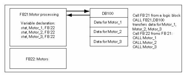
In this example, FB22 does not need its own instance data block, since its instance data are saved in the instance data block of the calling FB.
