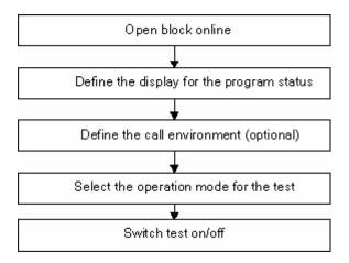
To set breakpoints, and to execute the program in single-step mode, test operation mode must be set (see menu command **Debug > Operation**). These test functions are not possible in process operation mode.
