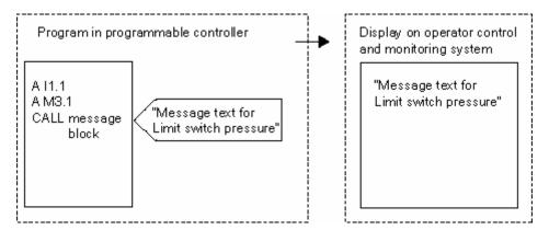
There is no cyclic query of the programmable controller. When the programmable controller signals a change, the corresponding message number is passed to the operator interface system and the corresponding message text is displayed. The message receives the time stamp from the programmable controller and can therefore be traced more exactly than with bit messaging.
