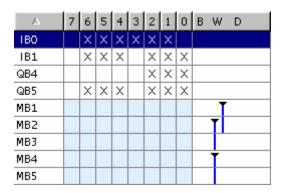
The first row shows the assignment of input byte IB 0. Inputs for address IB 0 are accessed directly (bit access). The columns "0", "1", "2", "3", "5", and "6" are identified with "X" for bit access.
