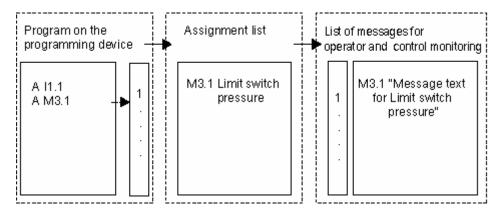
The operator interface system queries the programmable controller cyclically to see whether the message bit has changed or not. If the programmable controller signals a change, the corresponding message is displayed. The message receives the time stamp from the operator interface system.
