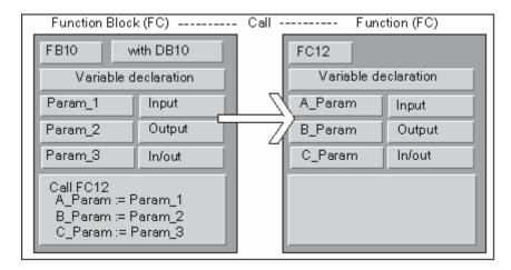
STEP 7 restricts the assignment of the formal parameters of an FB to the formal parameters of an FC. You cannot, for example, assign parameters of the parameter type as actual parameters. The following table shows the permitted data types  $(\bullet)$  when an FB calls an FC.
