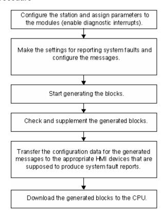
The messages are sent by means of the standard message path ALARM\_S/SQ to CPU Messages on the programming device or to the connected HMI devices. The sending of message to an HMI device can be deselected.
