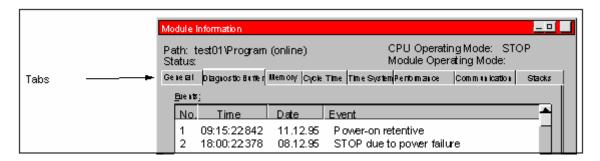
The names of the tab cards are shown on tabs along the top edge of the dialog box. To bring a particular tab card to the foreground, you simply click on its tab.
