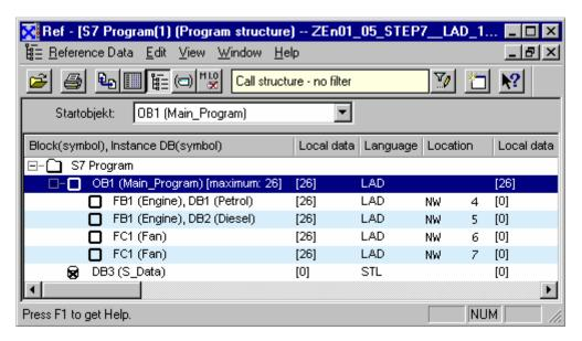
If the program structure is to be created for all organization blocks (OB) and OB1 is not in the S7 user program, or if a starting block was specified which is not present in the program, you are automatically prompted to specify another block for the program structure root.
