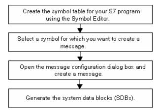
During processing, the signals for which you have configured messages are checked asynchronously to your program. The checks take place at the configured time intervals. The messages are displayed on the assigned display devices.
