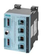
SCALANCE X201-3PIRT PRO; managed IE IRT Switch Degree of protection IP65/67; 1x 10/100 Mbit/s Push Pull RJ45 port; 3x 100 Mbit/s Push-pull SCRJ port; Error signaling contact with set pushbutton; Redundant power Supply; PROFINET IO device; network management; Redundancy Manager integrated, incl. electron. manual on CD-ROM, C-PLUG optional.
