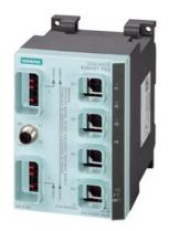
SCALANCE X204IRT PRO, managed IE IRT switch with degree of protection IP65/67, 4x 10/100 Mbit/s Push-pull RJ45 ports, error signaling contact with set push-button; redundant power supply; PROFINET IO device, network management, Redundancy Manager integrated, incl. electron. manual on CD-ROM, C-PLUG optional.
