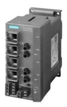
\*\*\*\*\*\*\*\*\*\*\* spare part \*\*\*\*\*\*\*\* SCALANCE X204-2TS; managed IE switch; 4x 10/100 Mbit/s RJ45 ports; 2x 100 Mbit/s multimode BFOC; LED diagnostics; error signaling contact with set push-button; redundant power supply; PROFINET I/O device; network management; Redundancy Manager integrated, incl. electron. manual on CD-ROM, C-PLUG optional.
