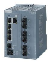
SCALANCE XB205-3 managed Layer 2 IE switch 5x 10/100 Mbit/s RJ45 ports 3x MM FO ST port 1x console port, diagnostics LED redundant power supply; IEC 62443-4-2 certified; temperature range 0 °C to +60 °C; DIN-rail mounting; default PROFINET.
