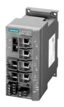
\*\*\*\*\*\*\*\*\*\* spare part \*\*\*\*\*\*\*\* SCALANCE X306-1LD FE managed IE switch, 6x 10/100 Mbit/s RJ45 ports, 1x 100 Mbit/s SC port single-mode; LED diagnostics, error signaling contact with select/set pushbutton, PROFINET IO device, network management, integrated redundancy manager, office features (RSTP, VLAN, IGMP,...) C-plug in scope of delivery .
