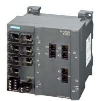
\*\*\*\*\*\*\*\*\*\* spare part \*\*\*\*\*\*\*\* SCALANCE X307-3LD, managed plus IE switch, 3x 1000 Mbit/s SM SC 7x 10/100 Mbit/s RJ45 ports, LED diagnostics, error-signaling contact with select/set pushbutton, PROFINET IO device, network management, integrated redundancy manager, office features (RSTP, VLAN, IGMP,...) C-plug in scope of delivery .
