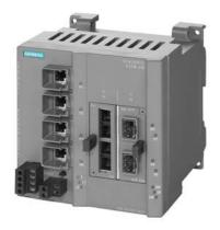
\*\*\*\*\*\*\*\*\* spare part \*\*\*\*\*\*\* SCALANCE X308-2M; managed IE switch, compact; 4x 10/100/1000 Mbit/s for RJ45 ports electrical; 2x 100/1000 Mbit/s for 2-port media modules, electrical or optical; LED diagnostics; error signaling contact; select/set pushbutton; PROFINET IO device; network management; Integrated redundancy manager; office features (RSTP, VLAN, IGMP,...); C-PLUG in scope of supply.
