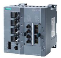
\*\*\*\*\*\*\*\*\* spare part \*\*\*\*\*\*\*\* SCALANCE X308-2M PoE; managed IE switch, compact; 4x 10/100/1000 Mbit/s for RJ45 ports electrical with PoE; 2x 100/1000 Mbit/s for 2-port media modules, electrical or optical; LED diagnostics, error signaling Contact with select/set pushbutton, PROFINET IO device, network management, Integrated redundancy manager, office features (RSTP, VLAN, IGMP,..) C-plug in scope of supply.
