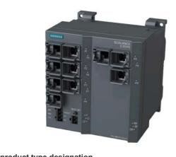
SCALANCE X310FE, managed plus IE switch, 10x 10/100 Mbit/s RJ45 ports, LED diagnostics, error-signaling contact with Select/set pushbutton, PROFINET IO Device, network management, integrated redundancy manager, Office features (RSTP, VLAN, IGMP,...) C-plug in scope of delivery .
