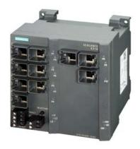
SCALANCE X310, managed plus IE switch, 3x 10/100/1000 Mbit/ and 7x 10/100 Mbit/s RJ45 ports LED diagnostics, error signaling Contact with select/set pushbutton, PROFINET IO device, network management, Integrated redundancy manager, office features (RSTP, VLAN, IGMP,...) C-plug in scope of supply.
