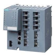
SCALANCE XM408-4C; managed modular IE switch;  $8x\ 10/100/1000\ Mbit/s\ RJ45$ ;  $4x\ 100/1000\ Mbps\ ST-/SC-$  pluggable as combo ports; in total 8 ports can be used; expandable to 24 ports electrical or optical; assembly: DIN rail/S7 mounting rail, PROFINET IO device; redundancy functions; office features (RSTP, VLAN, IGMP,..); C-PLUG in scope of supply; layer 3 with Key-Plug plug available .
