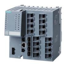
SCALANCE XM416-4C; managed modular IE switch; 16x 10/100/1000 Mbit/s RJ45; 4x 100/1000 Mbit/s SFP; contains 4 combo ports; in total 16 ports can be used; expandable to 24 ports electrical or optical; assembly: DIN rail/S7 mounting rail, PROFINET IO device; redundancy functions; office features (RSTP, VLAN, IGMP,..); C-PLUG in scope of supply; Layer 3 integrated;
