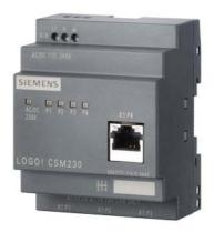
\*\*\*\*\*\*\*\* spare part \*\*\*\*\*\*\*\*\*\*\* LOGO! CSM 230 compact switch module of connection of a LOGO! (... 0BA7) and up to 3 further nodes to Industrial Ethernet with 10/100 Mbps; unmanaged switch, 4 RJ45 ports, 1x front port for diagnostics 115 ... 240 V AC/DC
