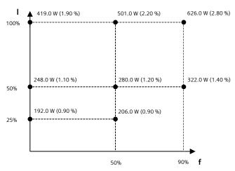
The percentage values show the losses in relation to the rated apparent power of the converter.
