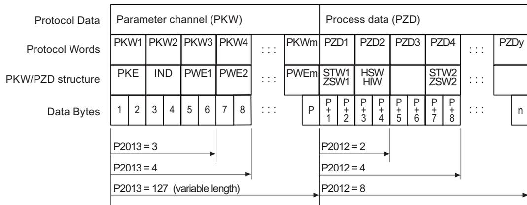
Figure 6-3 USS use data structure
