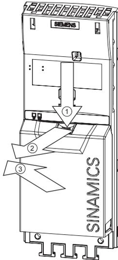
Figure 4-2 Removing the Control Unit terminal cover
