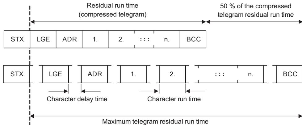
Figure 6-7 Residual Run Time and Character Delay Time
