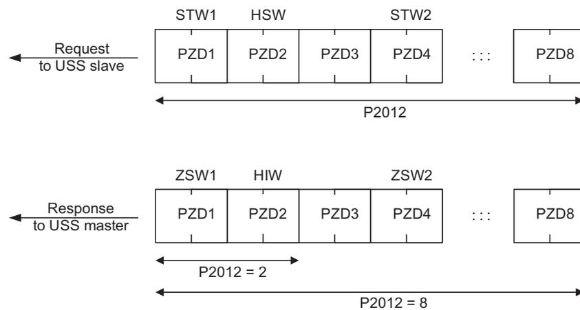
Figure 6-10 Process data channel
