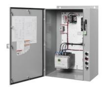
Enclosed soft starter, Controller 3RW44251BC34, Std duty rating 30Hp @460V, Std duty current rating 51A, Control voltage 115 AC, Combination type, 100A fusible disconnect, Enclosure NEMA type 1, Indoor general purpose use
