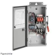
Slim Line Pump Control Panel NEMA size 1 Three phase full voltage Solid-state overload relay OLR amp range 3-12A 460VAC 60Hz Coil 30A fusible disconnect 30A/600V fuse clip 1NC / 1NO auxiliary contacts HOA Sel. Sw. <(>&<)> Start/Stop 3-point power terminal block 3-point control terminal block 3-point ground lug Enclosure NEMA type 3/3R Weather proof outdoor
