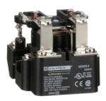
Power Relay, Type C, 1.5HP, 30A resistive at 300VAC, DPDT, 2 normally open and 2 normally closed contact, 120VAC coil
