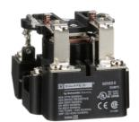
Power Relay, Type C, 2 hp, 30A resistive at 300VAC, DPDT, 2 normally open and 2 normally closed contact, 277VAC coil
