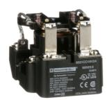
Power Relay, Type C, 2 hp, 30A resistive at 300VAC, DPDT, 2 normally open and 2 normally closed contact, 240VAC coil
