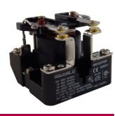
Power Relay, DPST, 2NO and 0NC, 2 hp, 30 A resistive at 300 VAC, 12 VAC coil
