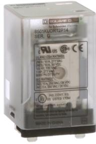
Plug in relay, Type KU, blade, 0.5 HP at 240 VAC, 10A resistive at 120 VAC, 8 blade, DPDT, 2 NO, 2 NC, 48 VDC coil
