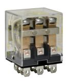
Plug in relay, Type R, miniature, 1 HP at 277 VAC, 15A resistive at 120 VAC, 11 blade, 3PDT, 3 NO, 3 NC, 240 VAC coil
