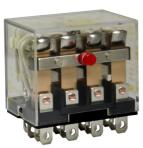
Plug in relay, Type R, miniature, 1 HP at 277 VAC, 15A resistive at 120 VAC, 14 blade, 4PDT, 4 NO, 4 NC, 24 VAC coil
