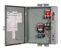
Pump control panel, Size 2, Three phase full voltage, Solid-state overload relay, OLR amp range 13-52A, 110-120/220-240VAC 60Hz coil, Standard type contactor, 60A fusible disconnect, 60A/600V fuse clip, HOA Sel Sw. <(>&<)> Start P.B., Enclosure NEMA type 3/3R, Weather proof outdoor use
