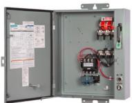
Pump control panel, Size 2, Three phase full voltage, Solid-state overload relay, OLR amp range 13-52A, 220-240/440-480VAC 60Hz coil, Standard type contactor, 60A fusible disconnect, 60A/600V fuse clip, HOA Sel Sw. <(>&<)> Start P.B., Enclosure NEMA type 3/3R, Weather proof outdoor use
