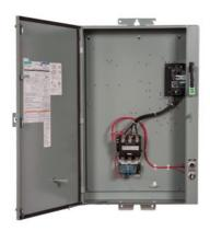
Pump control panel, Size 3, Three phase full voltage, Solid-state overload relay, OLR amp range 25-100A, 220-240/440-480VAC 60Hz coil, Standard type contactor, 100A circuit breaker, HOA Sel Sw. <(>&<)> Start P.B., Enclosure NEMA type 3/3R, Weather proof outdoor use
