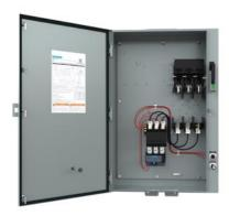
Pump control panel, Size 3 1/2, Three phase full voltage, Solid-state overload relay, OLR amp range 50-200A, 220-240/440-480VAC 60Hz coil, Standard type contactor, 200A fusible disconnect, 200A/600V fuse clip, HOA Sel Sw. <(>&<)> Start P.B., Enclosure NEMA type 3/3R, Weather proof outdoor use
