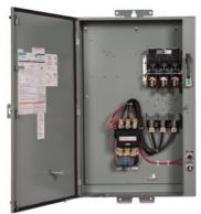
Pump control panel, Size 4, Three phase full voltage, Solid-state overload relay, OLR amp range 50-200A, 110-120/220-240VAC 60Hz coil, Standard type contactor, 200A fusible disconnect, 200A/600V fuse clip, HOA Sel Sw. <(>&<)> Start P.B., Enclosure NEMA type 3/3R, Weather proof outdoor use
