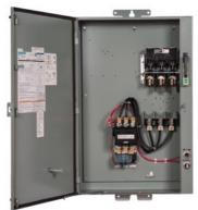
Pump control panel, Size 4, Three phase full voltage, Solid-state overload relay, OLR amp range 50-200A, 220-240/440-480VAC 60Hz coil, Standard type contactor, 200A fusible disconnect, 200A/600V fuse clip, HOA Sel Sw. <(>&<)> Start P.B., Enclosure NEMA type 3/3R, Weather proof outdoor use
