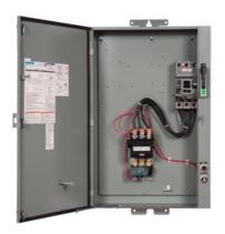
Pump control panel, Size 4, Three phase full voltage, Solid-state overload relay, OLR amp range 50-200A, 220-240/440-480VAC 60Hz coil, Standard type contactor, 150A circuit breaker, HOA Sel Sw. <(>&<)> Start P.B., Enclosure NEMA type 3/3R, Weather proof outdoor use
