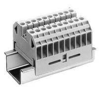
Through-type terminal thermoplast Screw terminal on both sides Terminal block 10-pole, beige with label 1...10 61mm, Sz. 2.5
