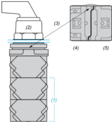
(1) It is possible to mount up to 3 levels of contacts blocks (maximum of 6 contacts blocks)
