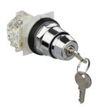
Selector switch, Harmony 9001K, metal, key switch, key active left, 30mm, key E10, 2 positions, Cam E, stay put, 1 CO pos 2
