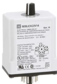
Timing Relay, Type JCK, plug In, off delay, adjustable time, 0.3 to 30 seconds, 10A, 240 VAC, 24 VAC/DC
