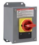
Manual Motor Switch, TeSys Vario, rotary handle, 25A, 3 pole, 10HP at 480V, metallic enclosure, UL Type 12
