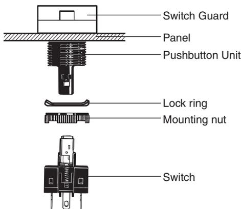
1. Insert the Case (Pushbutton Unit) into the Switch Guard.
