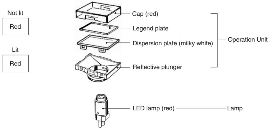
With colored illumination, the color of the lighted surface is white when the LED is not lit and the LED emits another color when it is lit.
