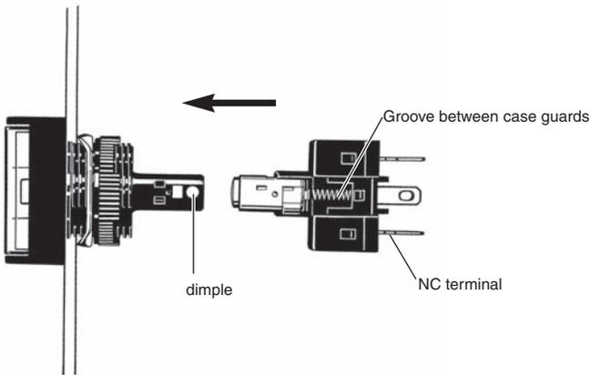
**Removing the Switch Unit**
