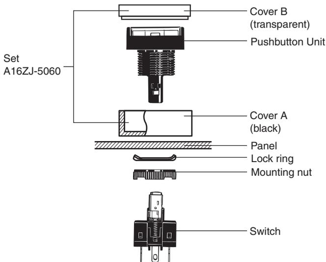
1. Separate the Dust Cover into 2 parts: cover A and cover B.
