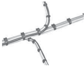
Sample cable tie installations
