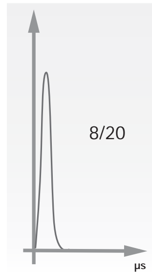
Type 2 Surge Arresters I_{max} : current wave
