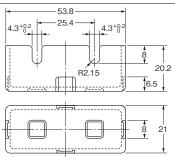
Note: The Cover has six thin, easy-to-separate portions for easy lead wire connections.
