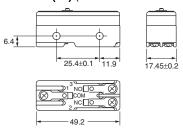
Note: 1. Appropriate terminal screw tightening torque: 0.78 to 1.18 N·m.
