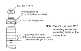
Note: Unless otherwise specified, a tolerance of  $\pm 0.4 \ \text{mm}$  applies to all dimensions.
