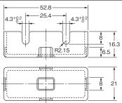
Note: The Cover has five thin, easy-to-separate portions for easy lead wire connections.
