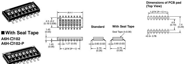
Note: 1. There is a tolerance of ±0.4 mm for each of the above dimensions unless otherwise specified in the diagrams.
