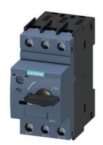
Circuit breaker size S0 for motor protection, Class 10 A-release 18...25 A N-release 325 A Screw terminal Standard switching capacity Multi-unit packaging Pack = 24 units
