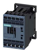
power contactor, AC-3e/AC-3, 7 A, 3 kW / 400 V, 3-pole, 110 V AC, 50 Hz / 120 V, 60 Hz, auxiliary contacts: 1 NO, spring-loaded terminal, size: S00, multi-unit packaging, pack = 32 units
