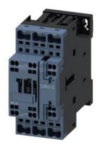
power contactor, AC-3e/AC-3, 32 A, 15 kW / 400 V, 3-pole, 110 V AC, 50 Hz / 120 V, 60 Hz, auxiliary contacts: 1 NO + 1 NC, spring-loaded terminal, size: S0, multi-unit packaging, pack = 18 units
