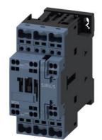
power contactor, AC-3e/AC-3, 25 A, 11 kW / 400 V, 3-pole, 110 V AC, 50 Hz / 120 V, 60 Hz, auxiliary contacts: 1 NO + 1 NC, spring-loaded terminal, size: S0, multi-unit packaging, pack = 18 units
